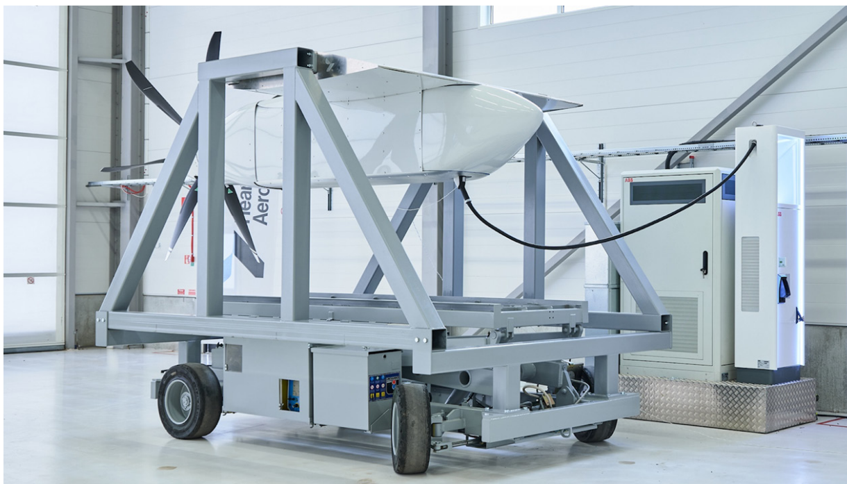
The picture shows the ES-19 powertrain demonstrator charging with a CC2 charger, at the Heart Aerospace hangar. Source: Heart Aerospace
