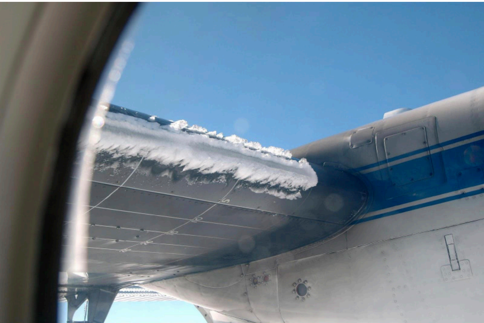
Illustration of icing on an aircraft wing. Source: NASA GRC
